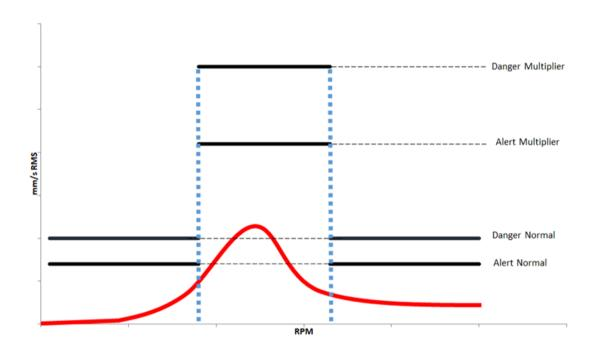
This function can be activated in 3 different ways (see manual "TDSP-Setup" - 4.7). When it is necessary to activate the Hardware contact, the TRIP Multiplier contacts must be closed towards GND in order to have the protection values of the machine multiplied by the values entered (exclusion of relays).
