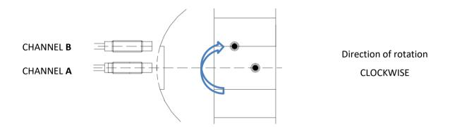
TD-2 monitoring system to be able to process in correct way the sense of rotation of the rotor needs necessary that the signal coming from channel A and the signal coming from channel B overlap for an instant. In the following image are reported the signals that the system must receive to check if the rotation is DIRECT or REVERSE.
