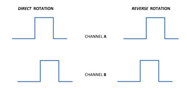
As it is possible to see from the image above, the TD-2 system in order to read the DIRECT rotation needs to receive first the channel A signal and then, superimposed, the channel B signal; for REVERSE rotation it needs to receive first the channel B signal and then, superimposed, the channel A signal.
